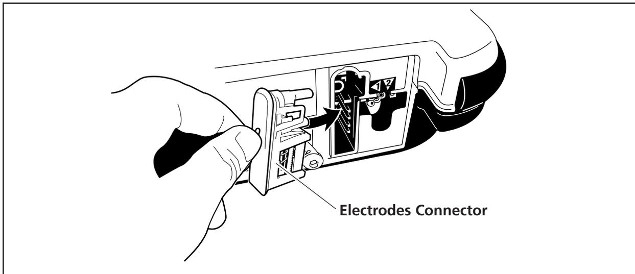
**Figure 3-24 Connecting the Electrodes to the AutoPulse**
