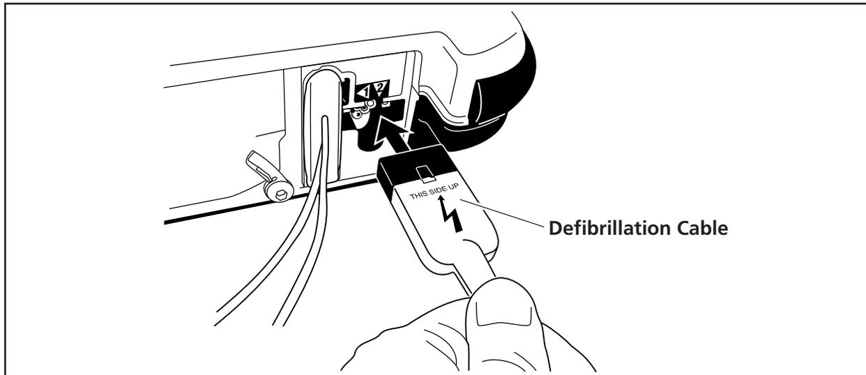
**Figure 3-25** Connecting the Defibrillation Cable to the AutoPulse
