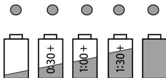
This is the **runtime indicator** that displays the estimated runtime of the *SurePower Battery Pack* in your defibrillator.
