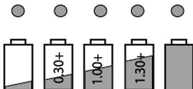
During the 2 seconds after you release the **Display** button, the runtime indicator displays battery capacity and will light five LEDs to indicate that the capacity is equal or close to that of a new battery.
